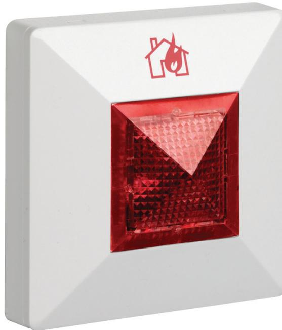
The intelligent addressable loop connected remote indicator (MRIAD) is designed to provide discreet remote indication, which is controlled by the intelligent addressable control panel, whilst providing the ability to monitor multiple sensors within an area thereby minimising wiring requirements.
